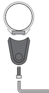
**Final mounting** Put the pump holder exactly on the tension plate and tighten the center screw with an allen key. If you like to change the adapter to a tube with a different diameter please use a new stainless strap (available as spare part).
