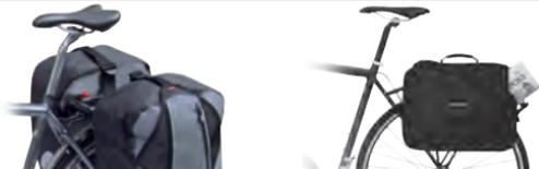
**Professional aluminium rail** for panniers with self adjusting locking mechanism for carriers Ø 8-16mm.
